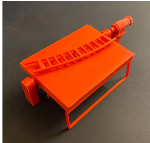
Figure 21: Switch Track 3D Printed Prototype Curved Track Side, Isometric View
