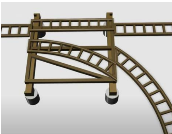
Figure 3: High Speed Live Transfer Switch Track
